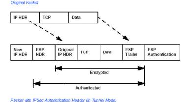
Figure C-3: Original packet and packet with IPSec ESP in Tunnel mode
